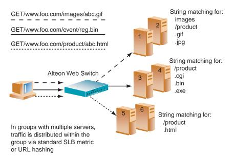
Figure 15-2 URL-Based Server Load Balancing
